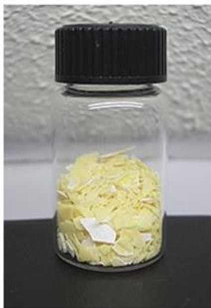
Figure 3. Photo of \text{Na}_2\text{S}\cdot 3\text{H}_2\text{O} solid, used in this work to prepare \text{Na}_2\text{S} solution
