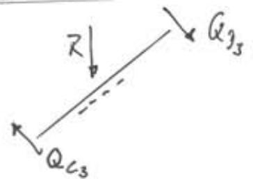
Stab 4:  $M_D = 0$ ;  $N = \text{const} = E_x = \underline{\underline{+2,121 \text{ kN}}}$
