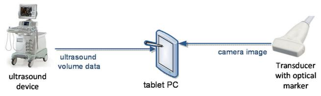
Fig. 1: Data flow for realizing AR ultrasound on tablet PCs
